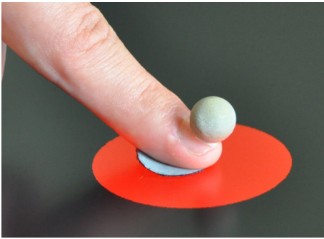
Figure 3. Implementing direct-touch with optical tracking. An optical marker is taped on the nail. A piece of soft fabric is taped underneath the finger to improve sliding.
